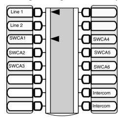
In this example, the call comes in on line 1 and automatically transfers to SWCA1 (the first free SWCA key).
